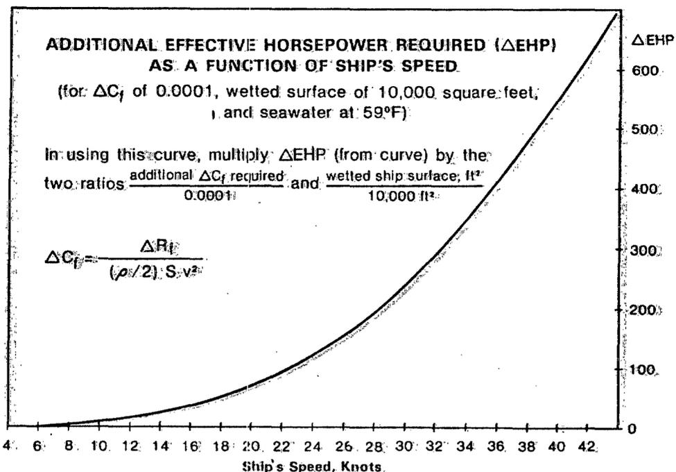
**Sample calculation:** To find the added effective horsepower (EHP) required for a guided missile cruiser (CG) at 30 knots when increasing  $\Delta C_f$  from 0.0006 to 0.0008.
