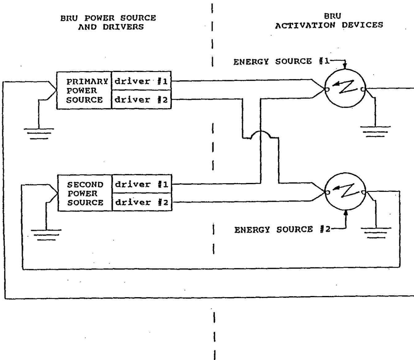
FIGURE 1. Wiring schematic to achieve primary and secondary release.
