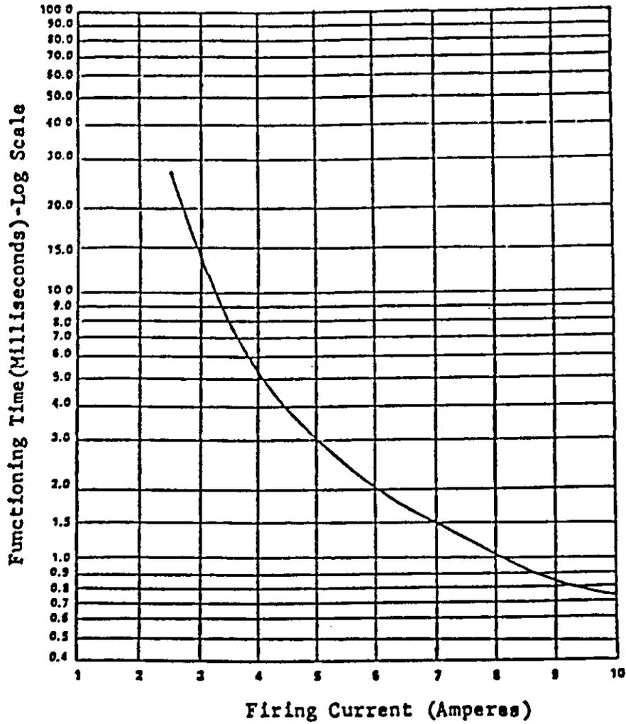
FIGURE 2. CCU-43/B, CCU-44/B, CCU-45/B cartridges functioning time vs applied current.
