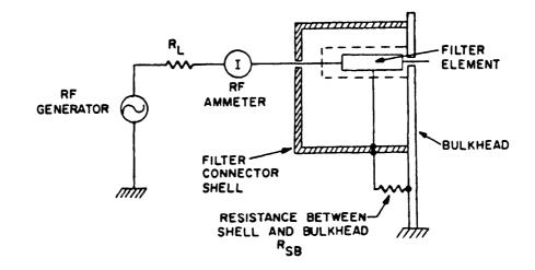
FIGURE 3. RF current test procedure.
