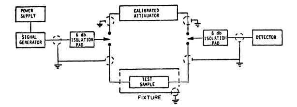
FIGURE 2. Attenuation measurement system.
