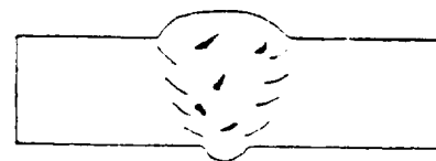
Cross section of weld
