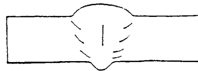
Lack of fusion at center of weld. Note complete penetration.
