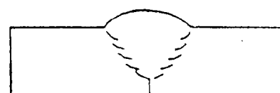
Cross section of weld
