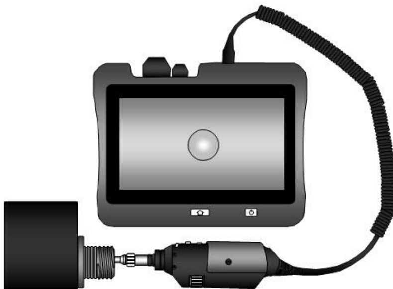
FIGURE 6M1-2. Example fiber optic video inspection system.
