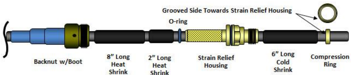
FIGURE 5A2-9. Strain relief parts on the cable.
