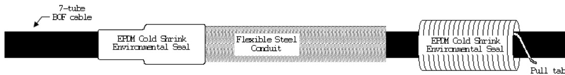
FIGURE 1C2-4. Half-finished splice.
