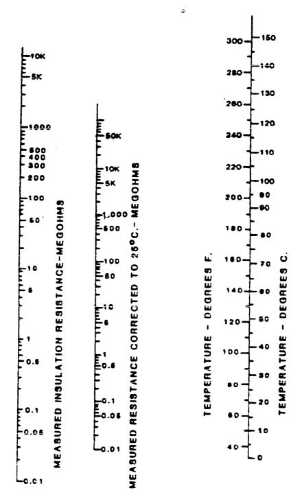
This nomograph is based on insulation resistance decreasing by one-half for each  $15^{\circ}\text{C}$  increase in temperature.
