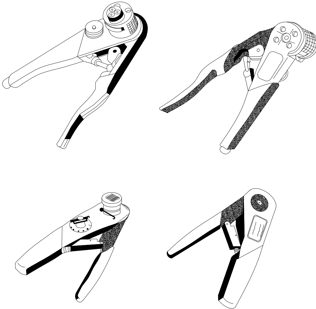
ILLUSTRATION 4 MIL-DTL-22520 CRIMPING TOOLS
