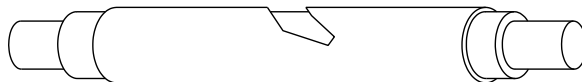
ILLUSTRATION 2. REPAIR STEP 1. TRIM LOOSE OR FRAYED PARTS OF CONDUCTOR INSULATION PROTECTIVE COVER.
