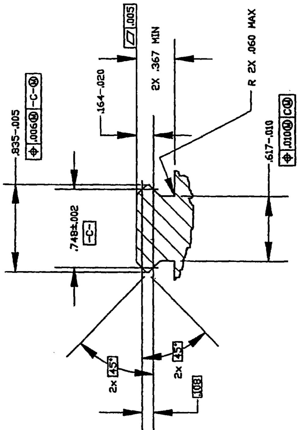
FIGURE 1. ACCESSORY MOUNTING RAIL PROFILE
