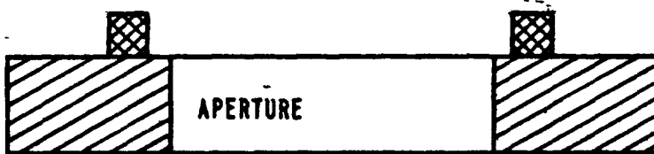
B. HELD IN PLACE BY SOLDERING (AMOUNT OF SOLDER USED MUST BE CAREFULLY CONTROLLED TO PREVENT ITS SOAKING INTO THE GASKET)
