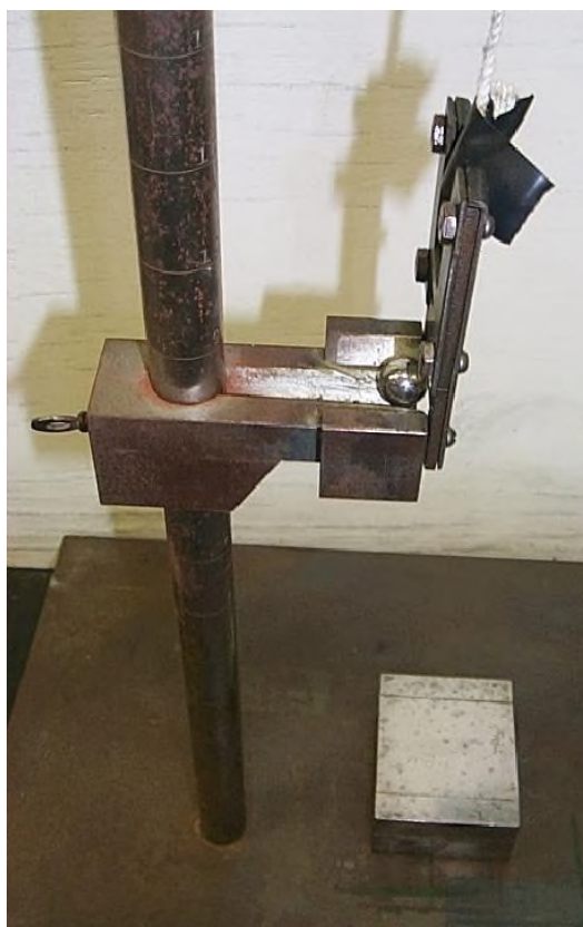
FIGURE 1. Ball Drop Impact Apparatus
