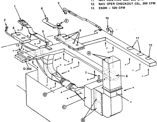
Figure 2. Ventilation system - Navigation Center 627 Class
