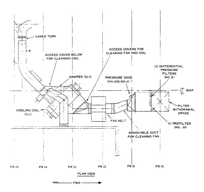
Figure 1. 598 Class navigation ventilation system equipment configuration (including ShipAlt 1142)
