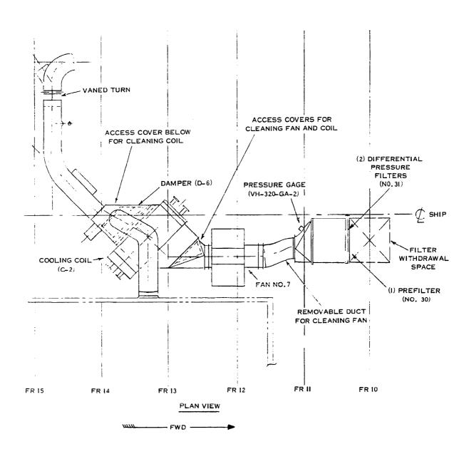
Figure 1. 598 Class navigation ventilation system equipment configuration (including ShipAlt 1142)
