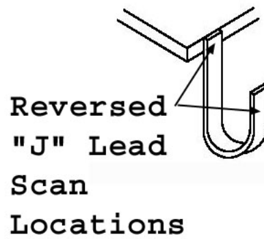
Figure 9-5. Scan Locations on Reversed J-Style lead
