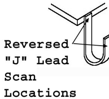
Figure 9-5. Scan Locations on Reversed J-Style lead
