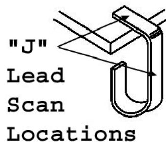
Figure 9-4. Scan Locations on J-Style lead
