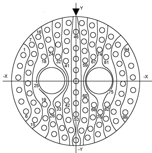
(Inactive for new design for MIL-DTL-38999. For new design, use arrangement no. 25-9.)
