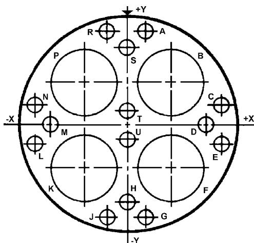
(Inactive for new design for MIL-DTL-38999. For new design, use arrangement no. 19-19.)
