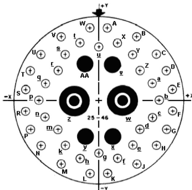
(Inactive for new design for MIL-DTL-38999. For new design, use arrangement no. 25-47.)
