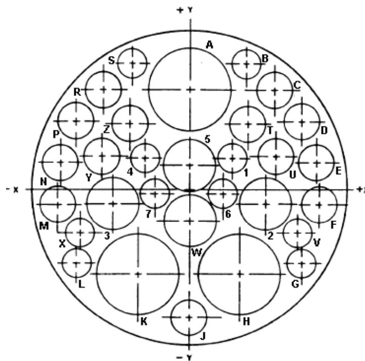
(This insert arrangement pattern is identical to arrangement 25-20, except this arrangement is designed to use MIL-DTL-38999/62 sealing boots with size 8 twinax contacts.)
