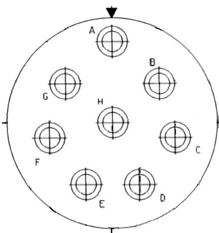
(Inactive for new design for MIL-DTL-38999. For new design, use arrangement no. 25-10.)
