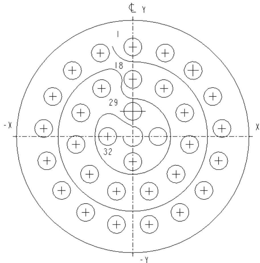
FIGURE 3. Insert arrangement, electrical connector, shell size 13 (series I, III, IV of MIL-DTL-38999, series I of MIL-DTL-27599, and series A of SAE-AS29600) – Continued.
