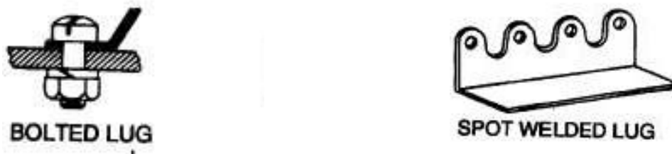
FIGURE 49. Grounding methods.
