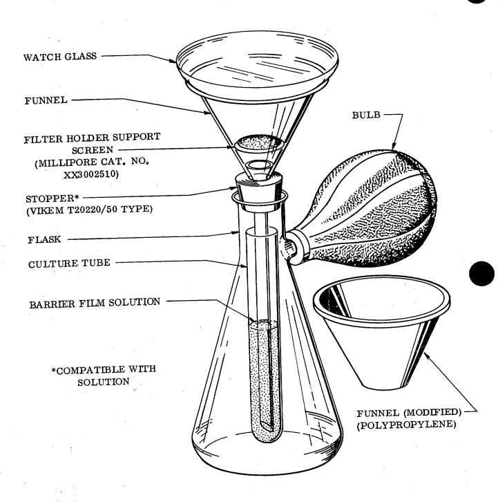
FIGURE 3. Screen-disc plain-funnel barrier film applicator/method III.
