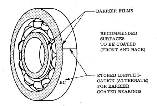
THE SEALS AND SHIELDS SHOULD BE DIPPED IN THE BARRIER FILM MATERIAL AND OVEN CURED BEFORE ASSEMBLY
