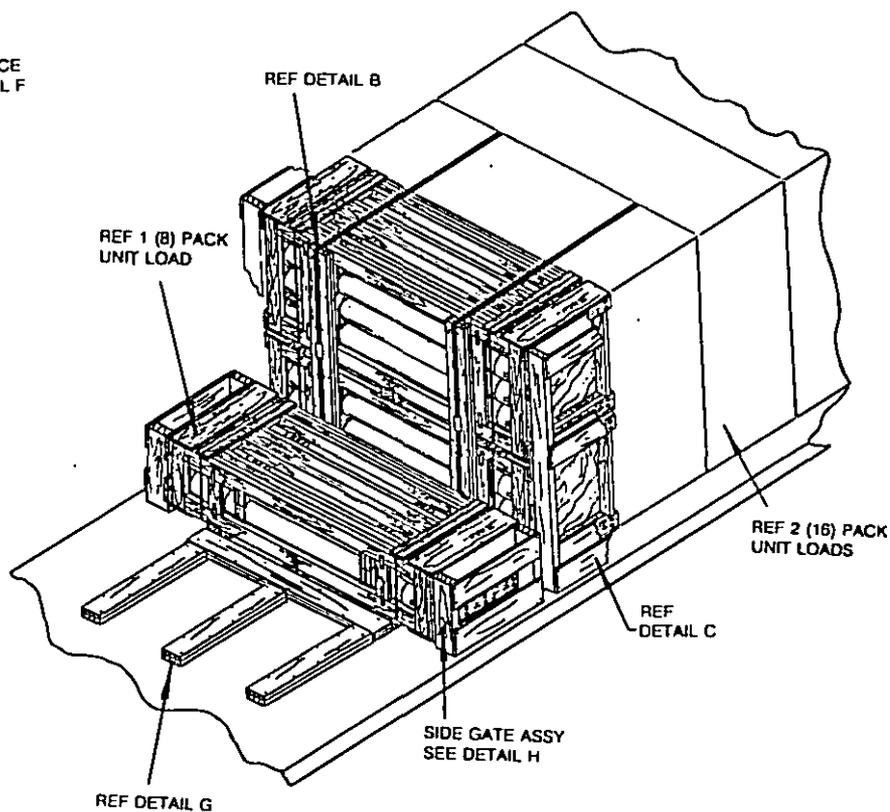
USED WHEN STACKING SINGLE 8, OR SINGLE 16 PACK, AGAINST DOUBLE 16 PACK UNIT LOAD.
