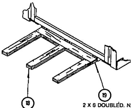
2 X 6 DOUBLED. (ALIGN WITH POST ON SKID) NAIL 1ST PC TO TRAILER FLOOR W/10-16d NAILS STAGGERED, NAIL 2ND PC TO 1ST IN LIKE MANNER.
