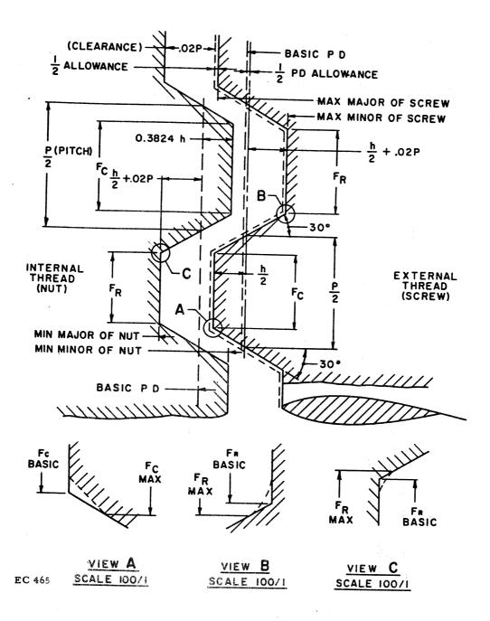
FIGURE 1. Basic dimensions - Class 2A and 2B threads. The dashed line indicates an allowance. Nut and screw threads have been separated for clarity.
