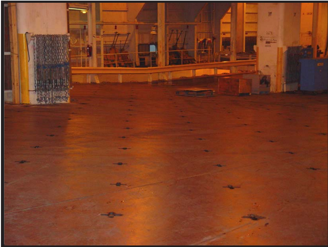
Figure 19. Typical FSS lashing pattern.
