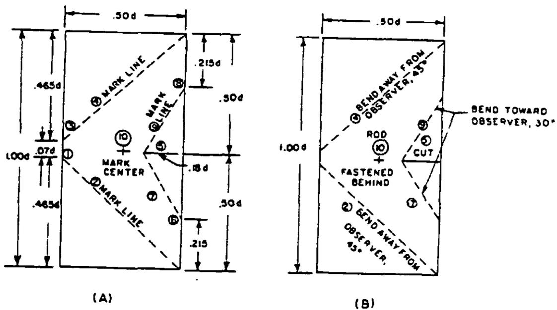
FIGURE C-1. Construction diagram for mode-stirrer.
