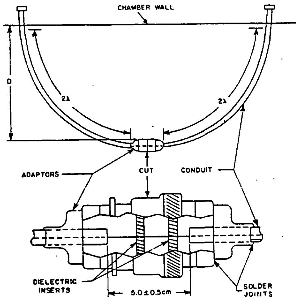
FIGURE 3. Preparation and installation of connector/conduit assembly.
