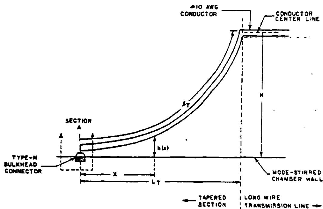
FIGURE B-2. Impedance matching taper.
