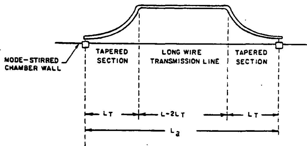
FIGURE B-1. Typical transmission line with taper.
