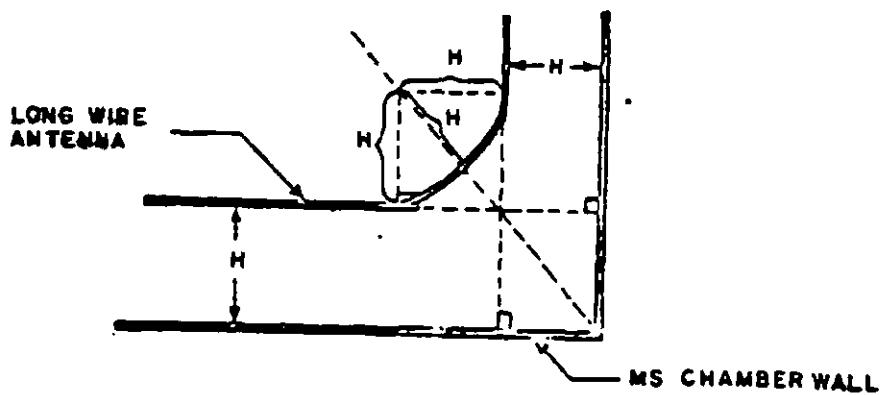
FIGURE A-2. Transmission line bend around corner.
