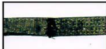
4. BROKEN OR WORN STITCHING
