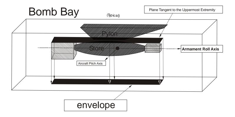
Note: The plane tangent to the uppermost extremity of the store parallel to the armament roll axis and parallel to the pitch axis of the aircraft.
