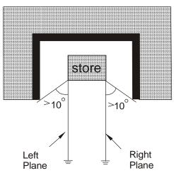
Note: Four planes tangent to the foremost, rearmost, right, and left extremities and parallel to the pitch axis of the store at an angle 10 degrees away from the vertical, expanding in the direction of the ground.
