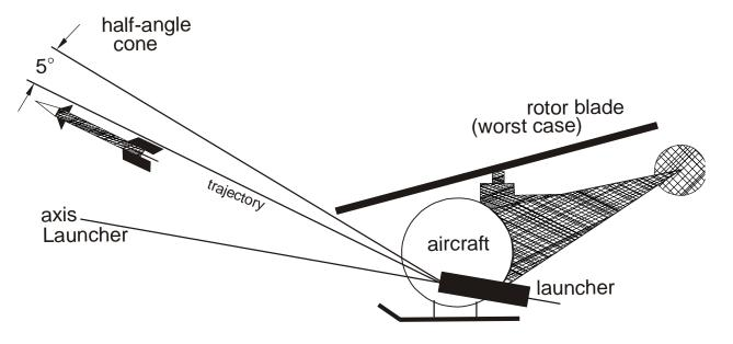
FIGURE 1. <u>Definition of a five-degree half-angle cone</u>
