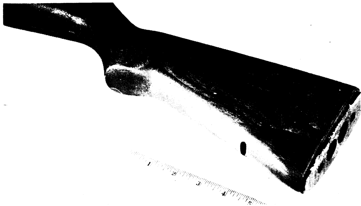
Patch exceeds size limits and extends into area where patching is not permitted
