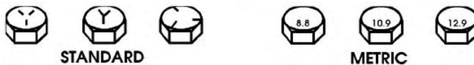
Figure 2. Capscrew Head Markings.
