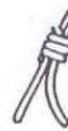
(p) “Third wire” - acceptable on AWG 18 through AWG 30 wire. Third wire must be uninsulated.
