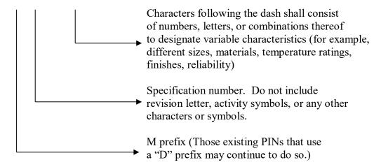
The above example also applies to MS sheet part numbers, except the prefix "MS" would be used instead of "M" and those PINS that use a "DS" prefix may continue to do so.
