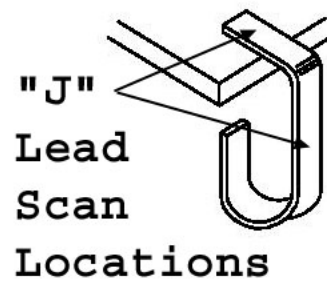
FIGURE 2037-3. Scan Locations on J-Style lead.
