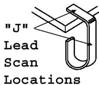
FIGURE 2037-3. Scan Locations on J-Style lead.
