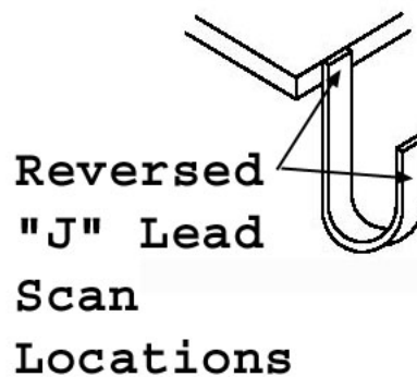
FIGURE 2037-4. Scan Locations on Reversed J-Style lead.
