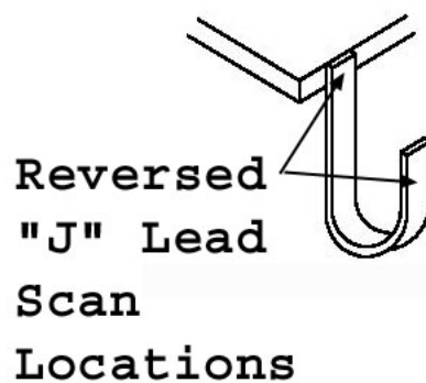
FIGURE 2037-4. Scan Locations on Reversed J-Style lead.
