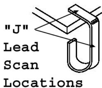
FIGURE 2037-3. Scan Locations on J-Style lead.
