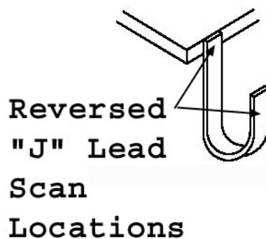
FIGURE 2037-4. Scan Locations on Reversed J-Style lead.
