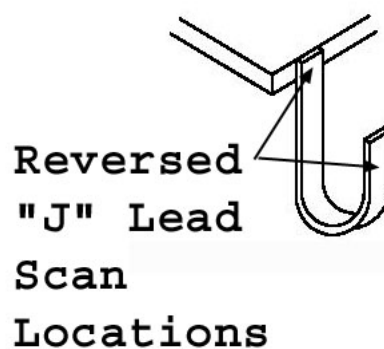
FIGURE 2037-4. Scan Locations on Reversed J-Style lead.
