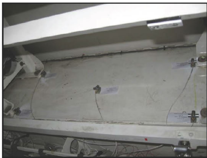
Figure 4. Transducer placement (input to missile rack).
