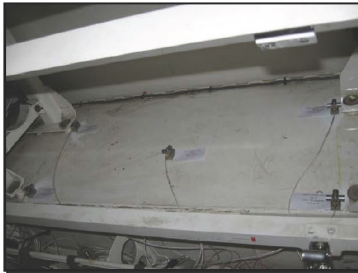
Figure 4. Transducer placement (input to missile rack).
