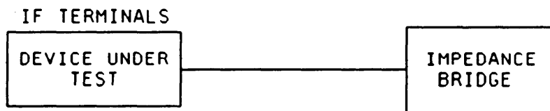
FIGURE 4116-2. Impedance bridge method.
