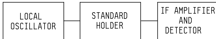
FIGURE 4121-1. Direct measurement method.
