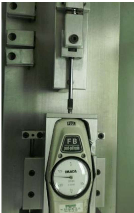
FIGURE 2038-1. Sample apparatus fixture with force measuring gauge.
