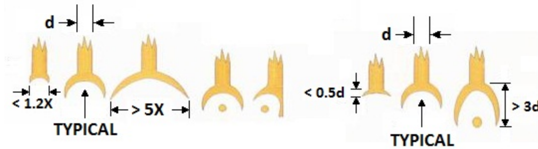
FIGURE 2072-23. Tailless bond dimensions.
