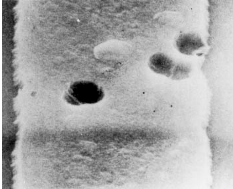
FIGURE 2077-20. General metallization voids at 5,000X (reject).
