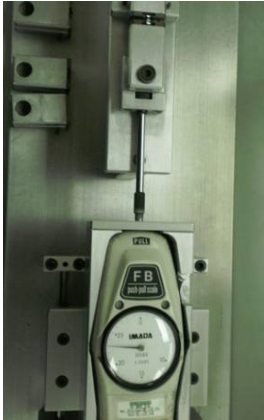
FIGURE 2038-1. Sample apparatus fixture with force measuring gauge.
