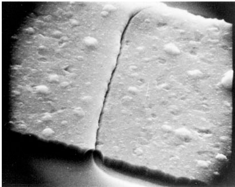
FIGURE 2077-9. Tunnel/cave at oxide step at 5,000X (reject).
