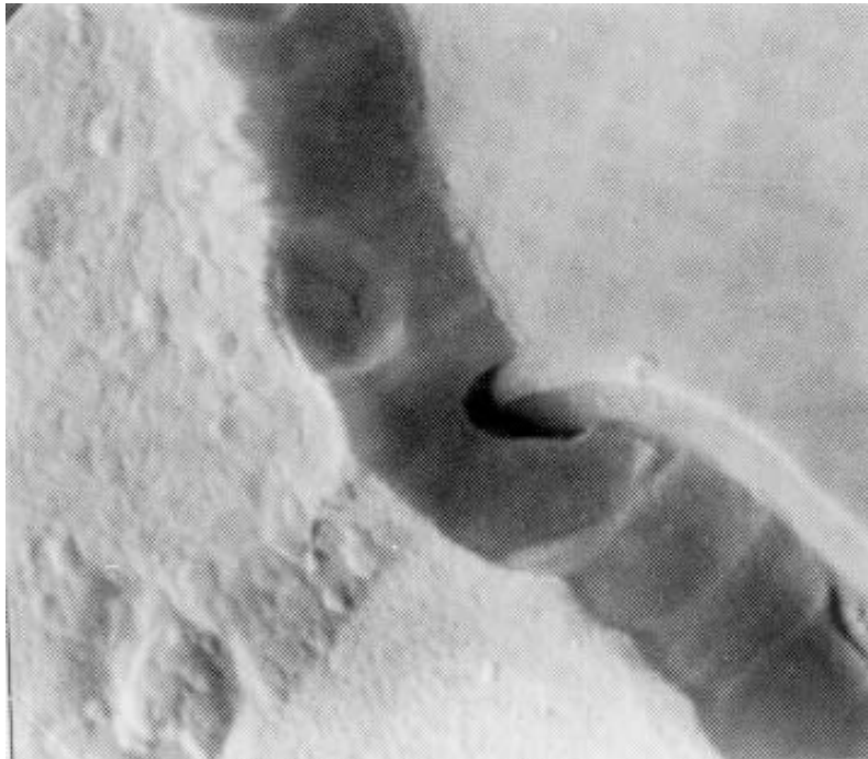
FIGURE 2077-8. Tunnel/cave at oxide step at 10,000X (accept).
