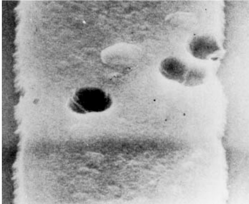
FIGURE 2077-20. General metallization voids at 5,000X (reject).
