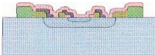
FIGURE 2072-9. Metallization misalignment, cross section view.
