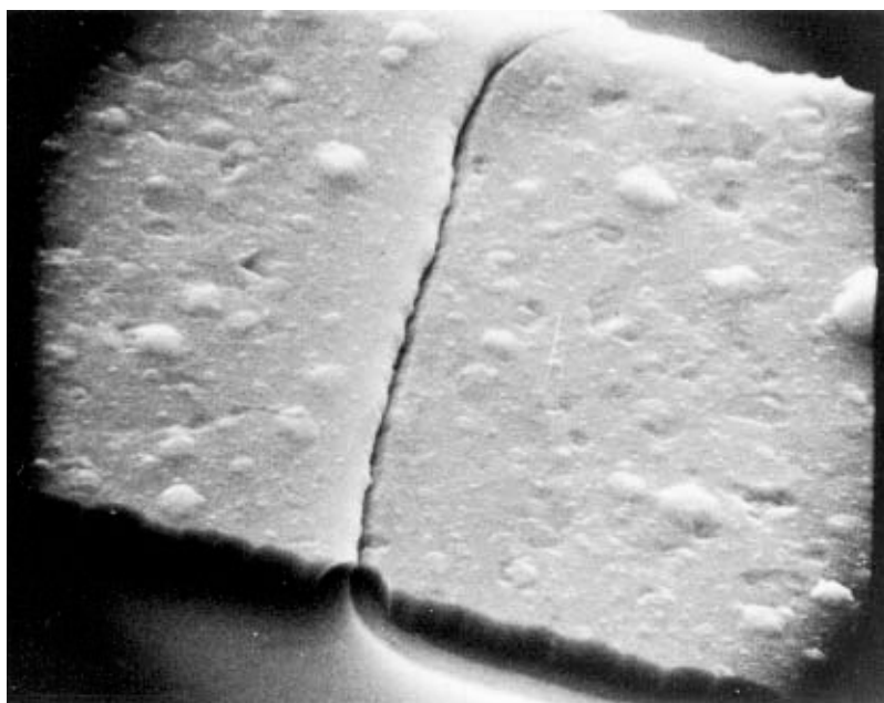
FIGURE 2077-9. Tunnel/cave at oxide step at 5,000X (reject).
