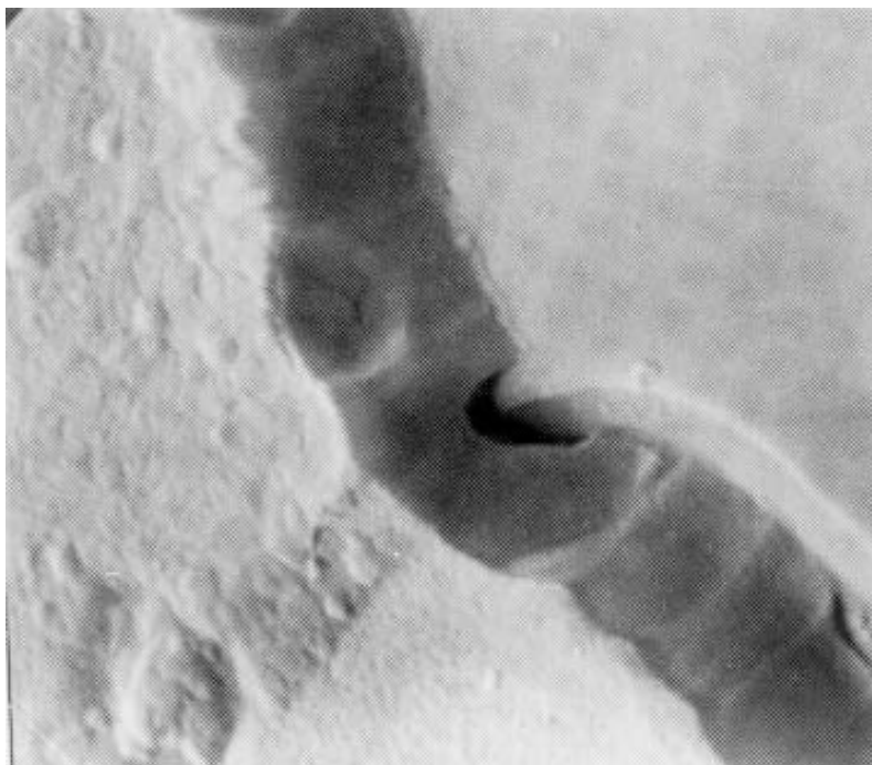
FIGURE 2077-8. Tunnel/cave at oxide step at 10,000X (accept).
