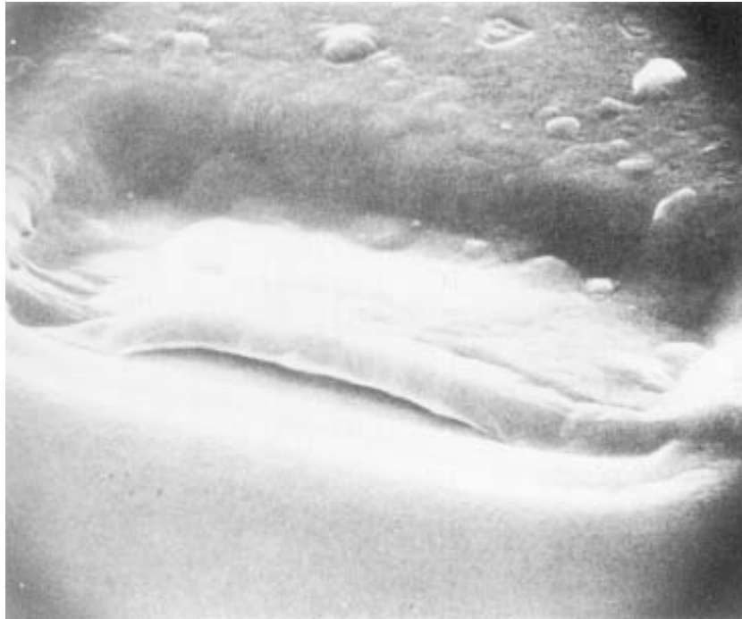
FIGURE 2077-18. Peeling or lifting of general metallization in contact window area at 5,000X (reject).
