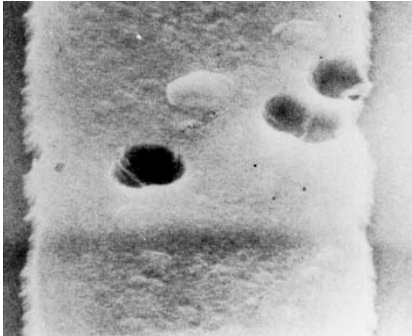
FIGURE 2077-20. General metallization voids at 5,000X (reject).
