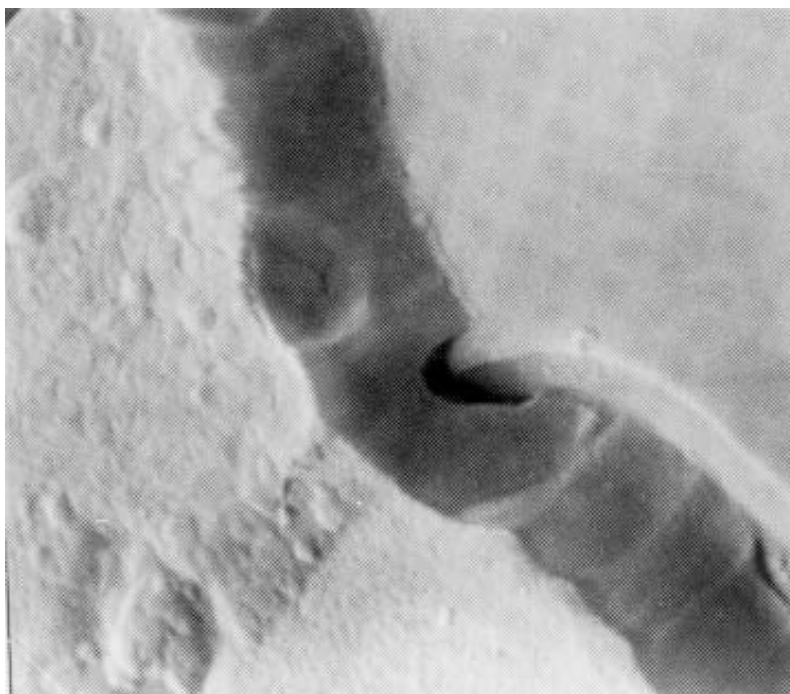
FIGURE 2077-8. Tunnel/cave at oxide step at 10,000X (accept).
