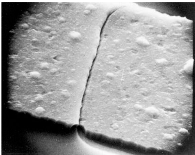
FIGURE 2077-9. Tunnel/cave at oxide step at 5,000X (reject).
