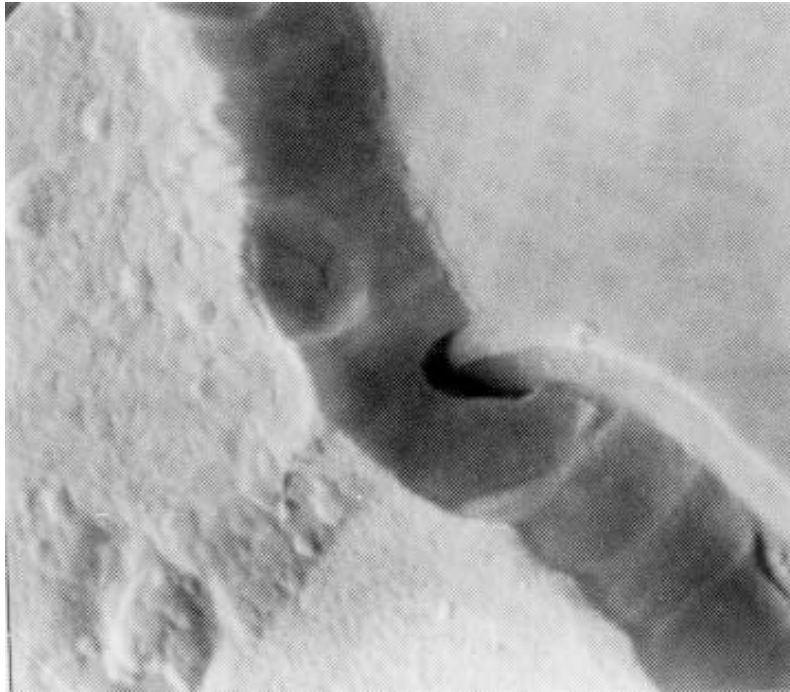
FIGURE 2077-8. Tunnel/cave at oxide step at 10,000X (accept).
