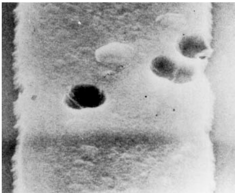
FIGURE 2077-20. General metallization voids at 5,000X (reject).
