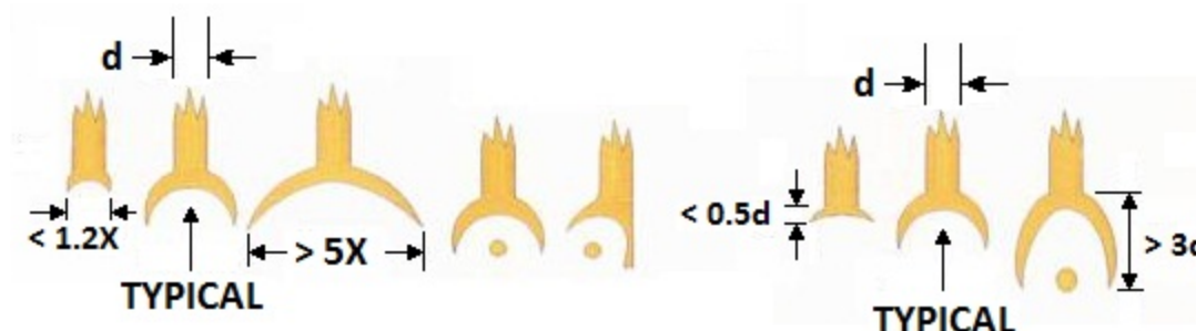
FIGURE 2072-23. Tailless bond dimensions.
