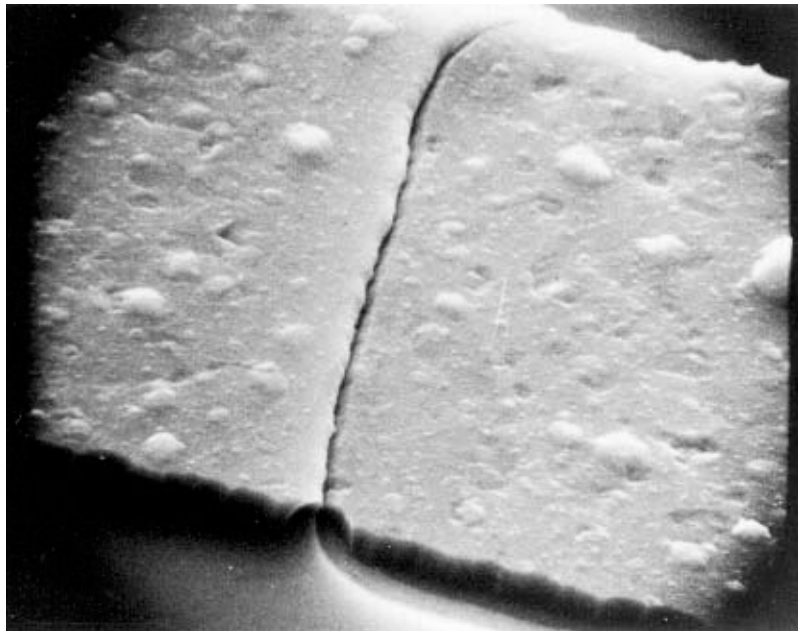
FIGURE 2077-9. Tunnel/cave at oxide step at 5,000X (reject).
