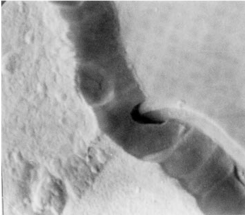
FIGURE 2077-8. Tunnel/cave at oxide step at 10,000X (accept).
