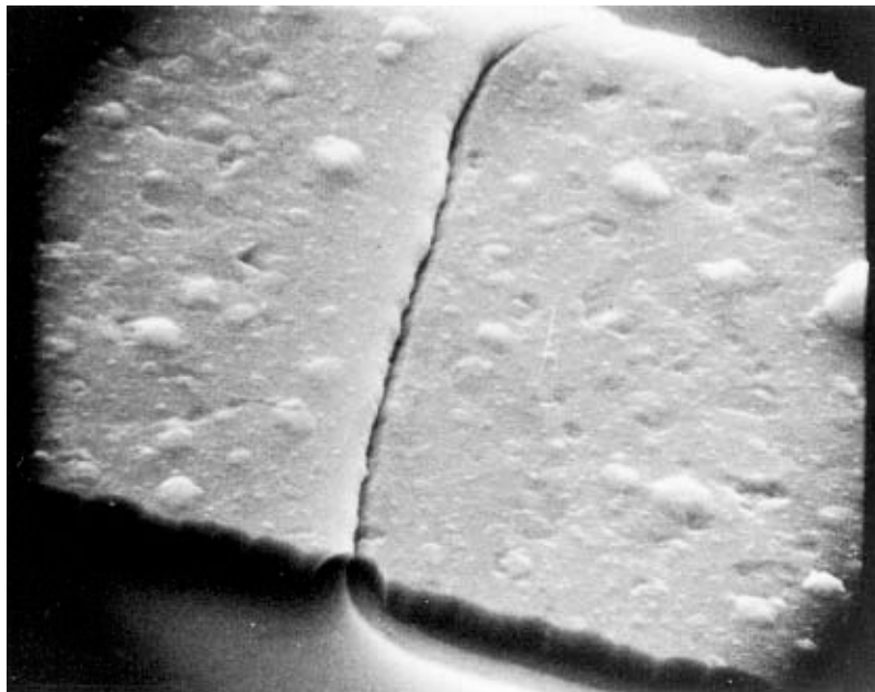
FIGURE 2077-9. Tunnel/cave at oxide step at 5,000X (reject).
