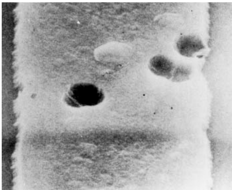
FIGURE 2077-20. General metallization voids at 5,000X (reject).
