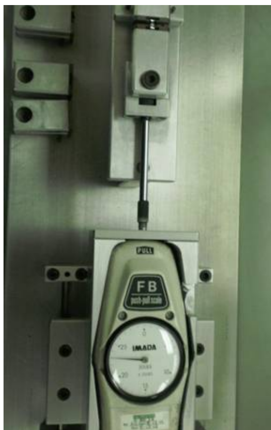
FIGURE 2038-1. Sample apparatus fixture with force measuring gauge.
