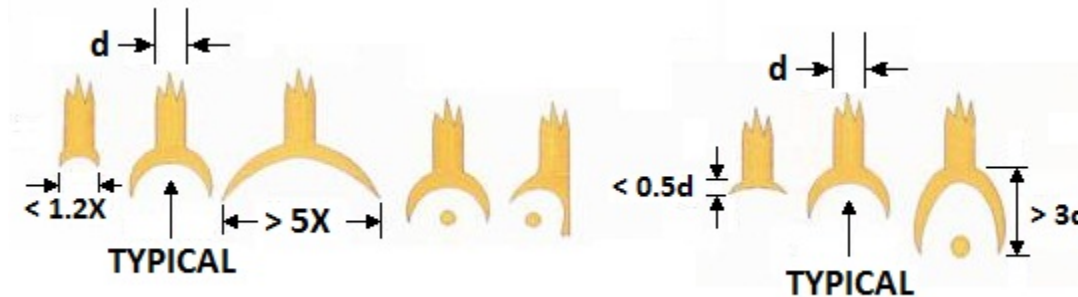
FIGURE 2072-23. Tailless bond dimensions.
