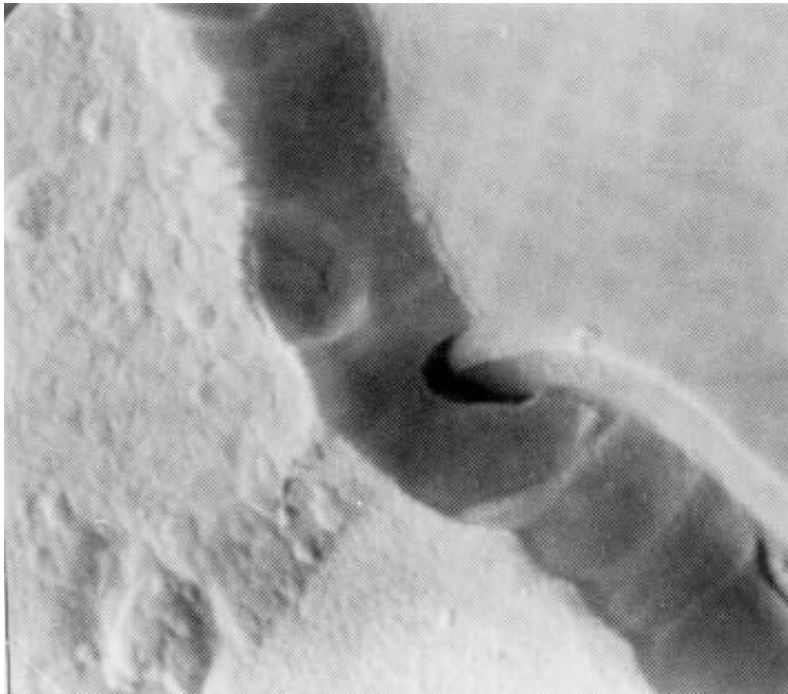
FIGURE 2077-8. Tunnel/cave at oxide step at 10,000X (accept).
