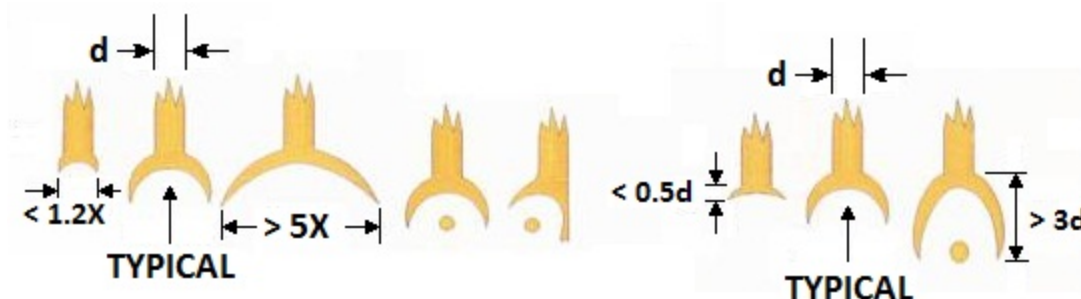
FIGURE 2072-23. Tailless bond dimensions.
