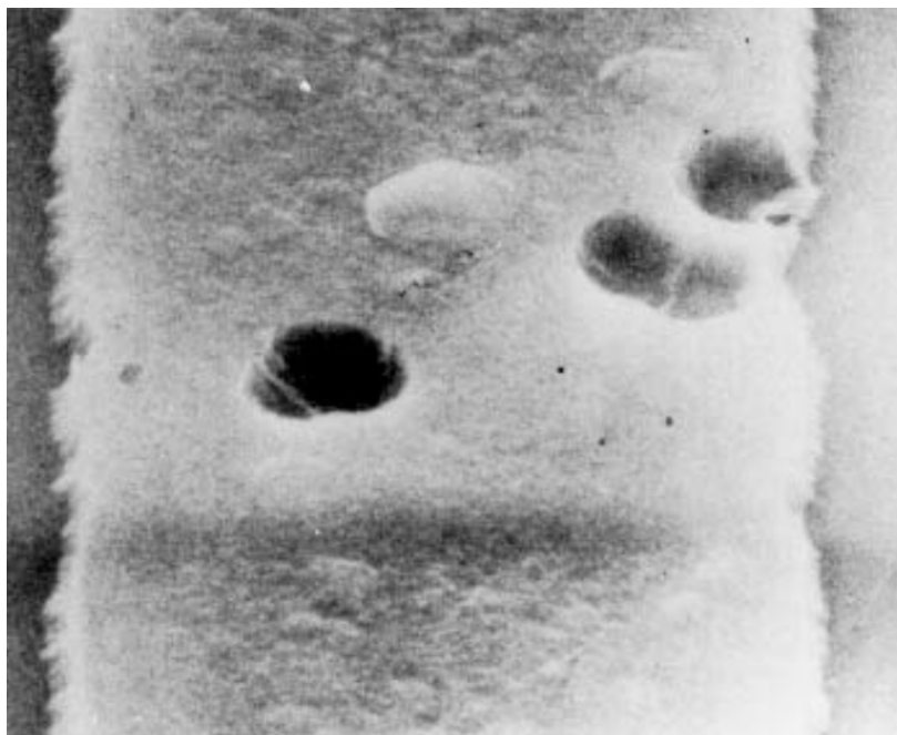
FIGURE 2077-20. General metallization voids at 5,000X (reject).
