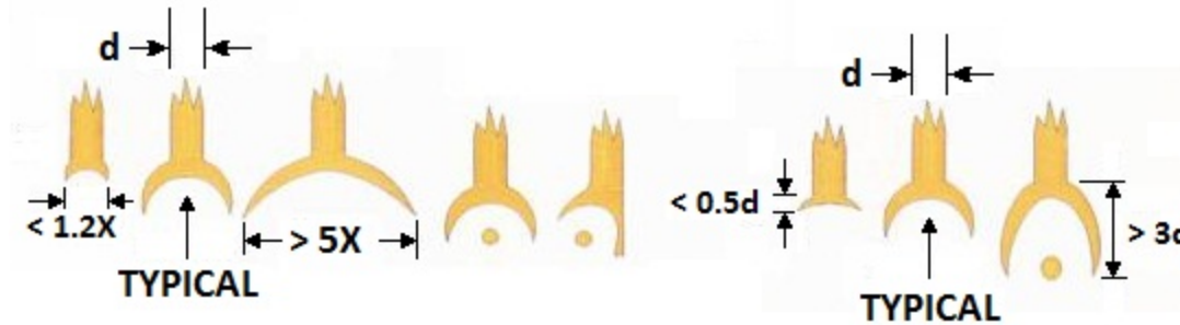
FIGURE 2072-23. Tailless bond dimensions.
