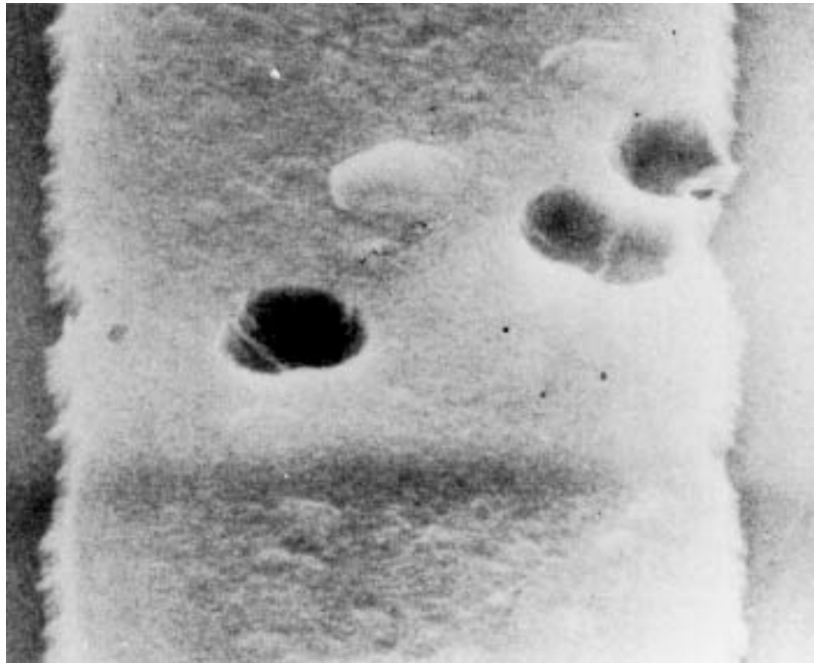
FIGURE 2077-20. General metallization voids at 5,000X (reject).
