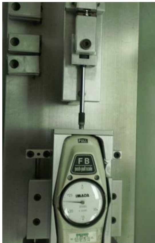
FIGURE 2038-1. Sample apparatus fixture with force measuring gauge.
