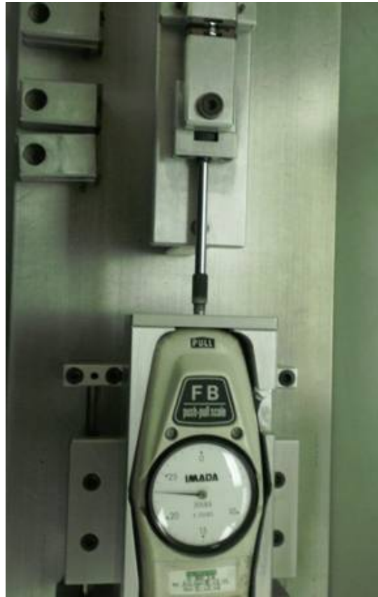
FIGURE 2038-1. Sample apparatus fixture with force measuring gauge.
