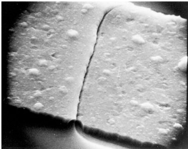
FIGURE 2077-9. Tunnel/cave at oxide step at 5,000X (reject).
