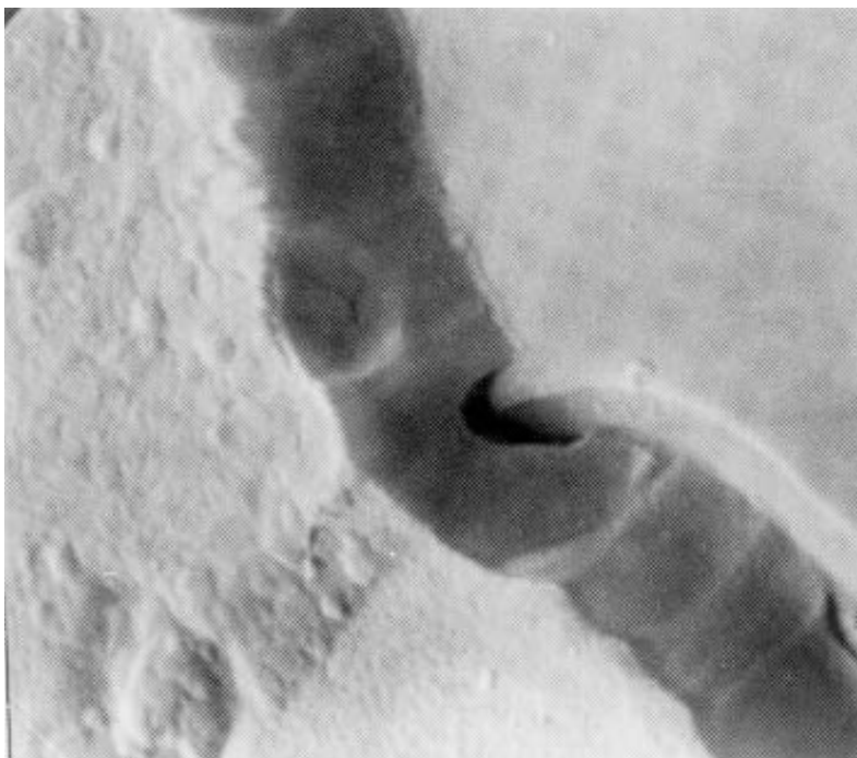
FIGURE 2077-8. Tunnel/cave at oxide step at 10,000X (accept).
