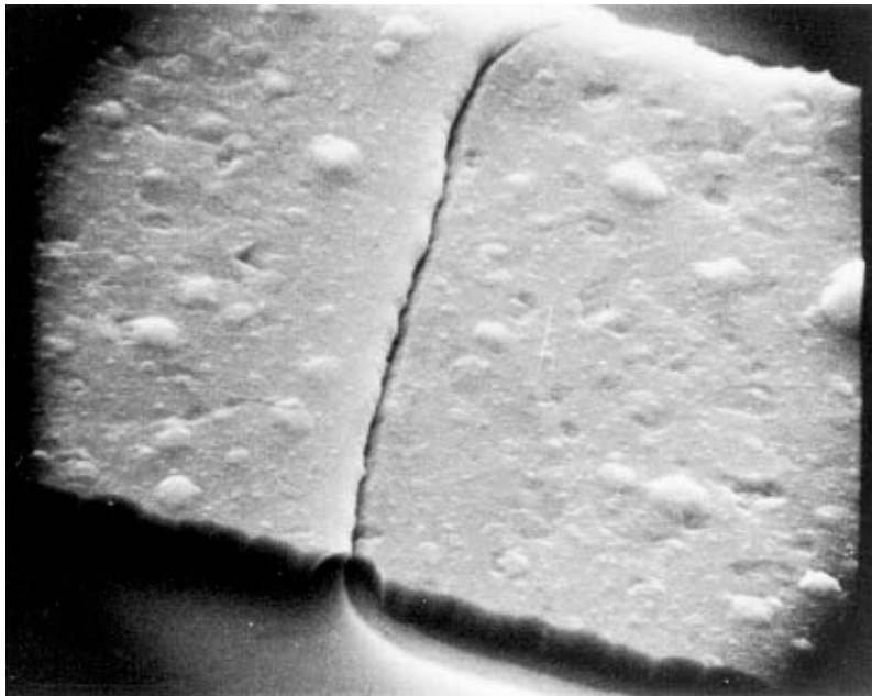
FIGURE 2077-9. Tunnel/cave at oxide step at 5,000X (reject).
