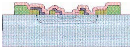
FIGURE 2072-9. Metallization misalignment, cross section view.
