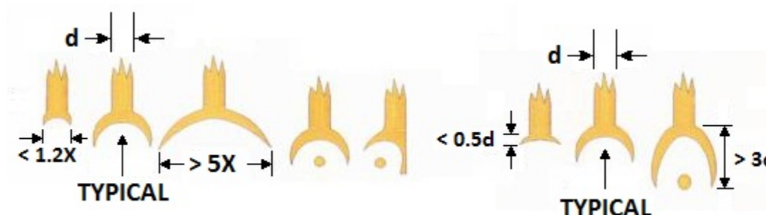
FIGURE 2072-23. Tailless bond dimensions.
