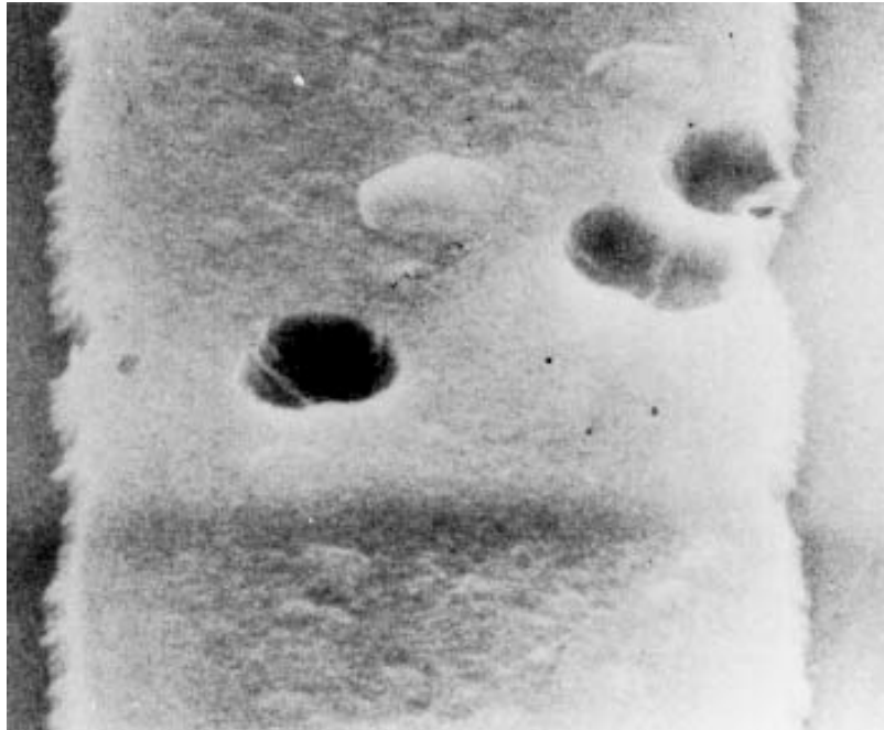
FIGURE 2077-20. General metallization voids at 5,000X (reject).
