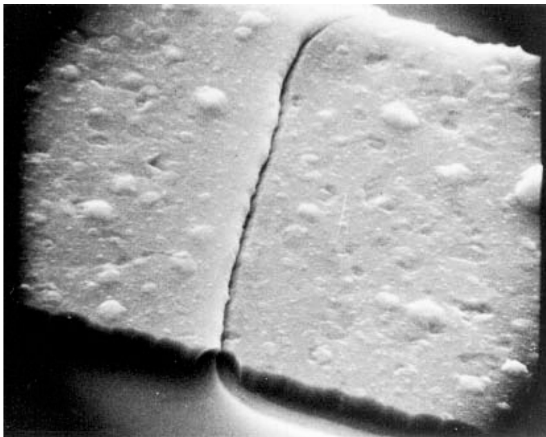
FIGURE 2077-9. Tunnel/cave at oxide step at 5,000X (reject).
