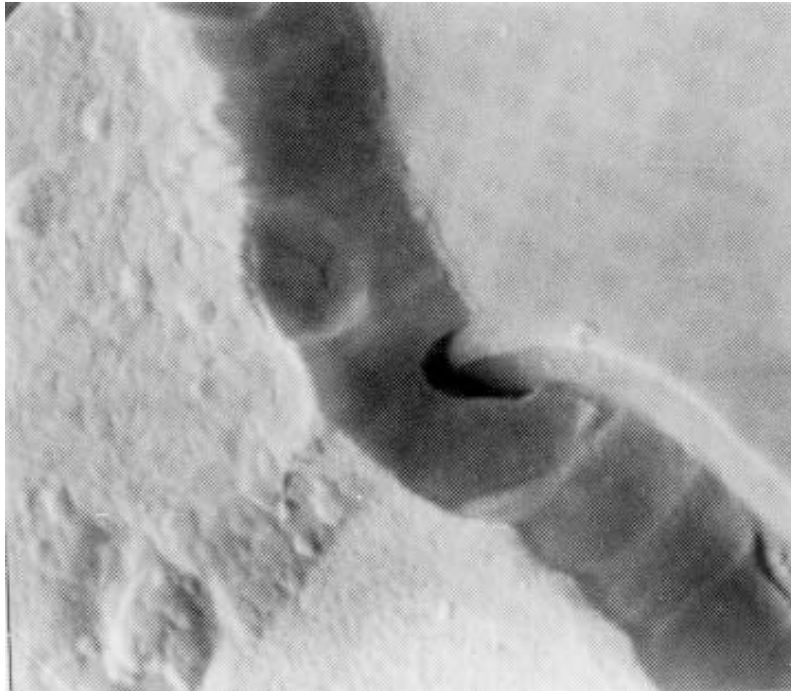
FIGURE 2077-8. Tunnel/cave at oxide step at 10,000X (accept).
