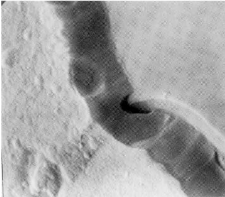
FIGURE 2077-8. Tunnel/cave at oxide step at 10,000X (accept).
