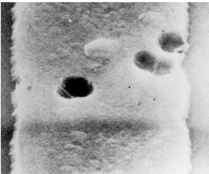
FIGURE 2077-20. General metallization voids at 5,000X (reject).
