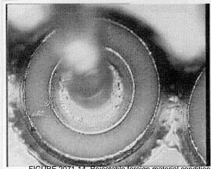
FIGURE 2071-14. Rejectable foreign material conditions continued.
