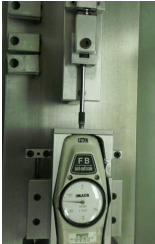
FIGURE 2038-1. Sample apparatus fixture with force measuring gauge.
