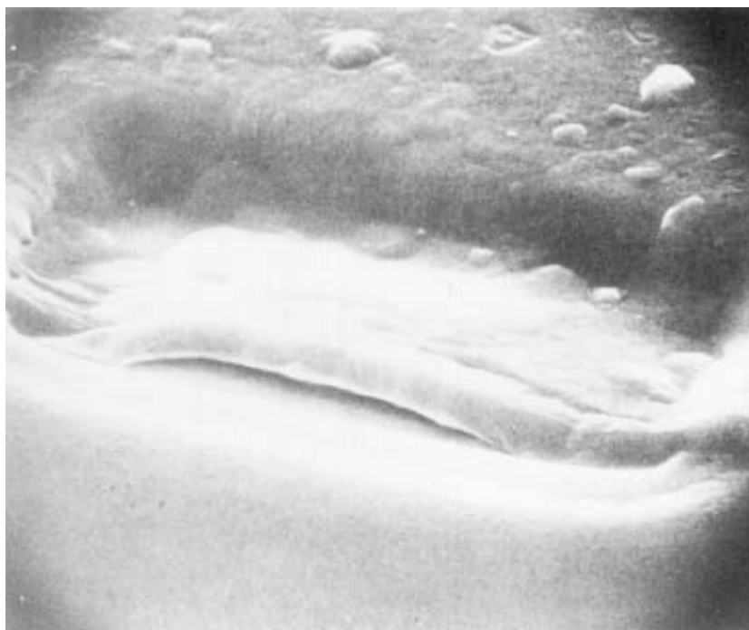
FIGURE 2077-18. Peeling or lifting of general metallization in contact window area at 5,000X (reject).
