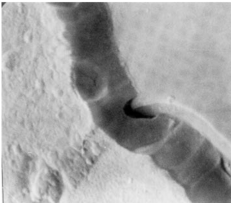
FIGURE 2077-8. Tunnel/cave at oxide step at 10,000X (accept).
