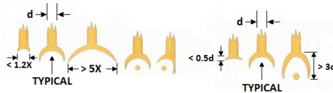
FIGURE 2072-23. Tailless bond dimensions.
