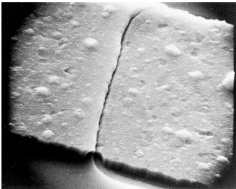
FIGURE 2077-9. Tunnel/cave at oxide step at 5,000X (reject).
