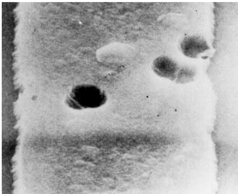
FIGURE 2077-20. General metallization voids at 5,000X (reject).
