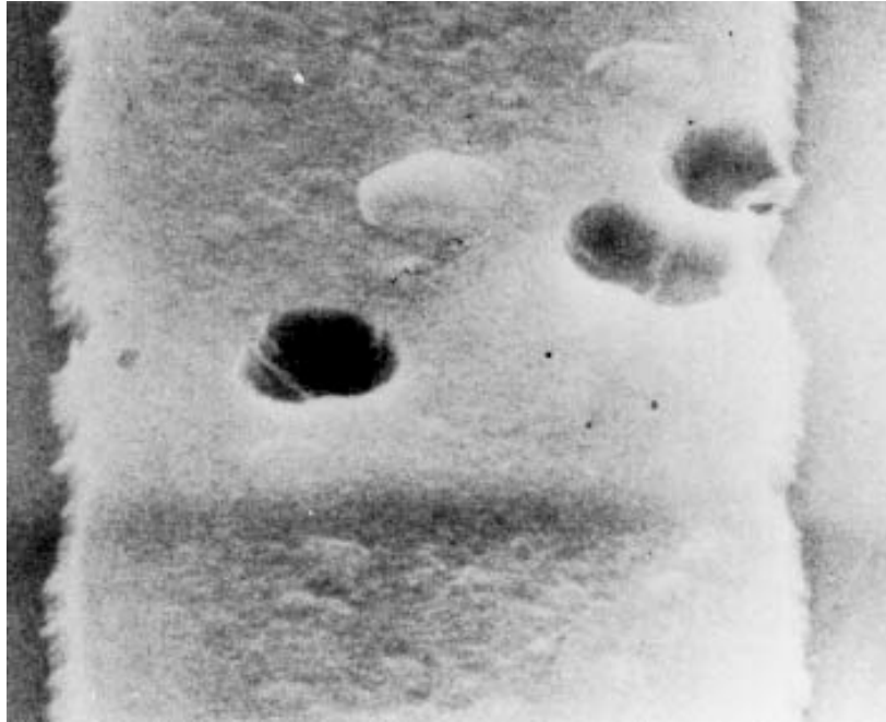
FIGURE 2077-20. General metallization voids at 5,000X (reject).
