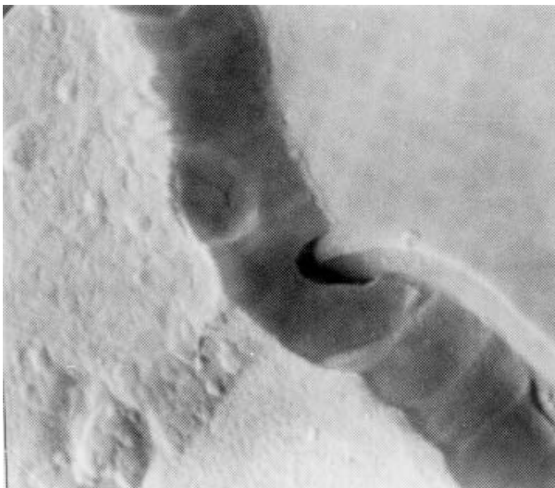
FIGURE 2077-8. Tunnel/cave at oxide step at 10,000X (accept).
