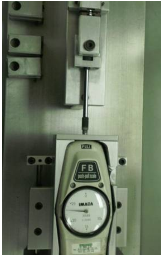
FIGURE 2038-1. Sample apparatus fixture with force measuring gauge.
