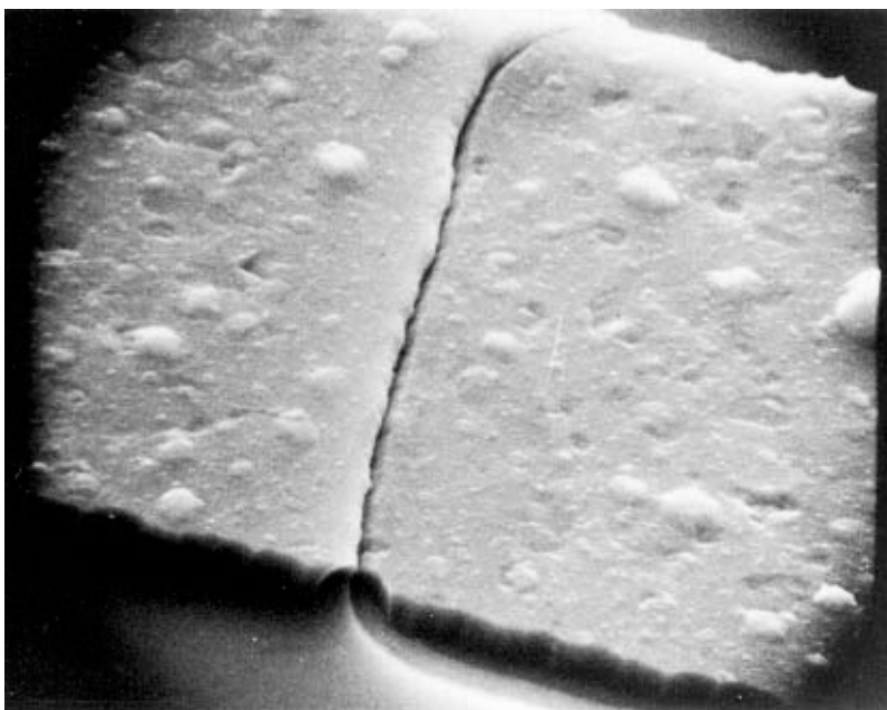
FIGURE 2077-9. Tunnel/cave at oxide step at 5,000X (reject).
