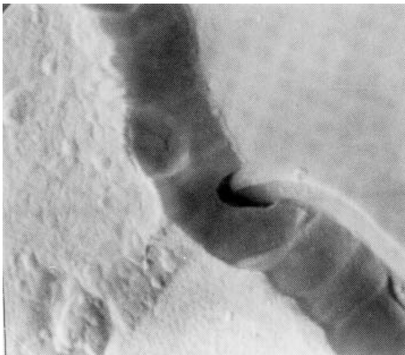
FIGURE 2077-8. Tunnel/cave at oxide step at 10,000X (accept).
