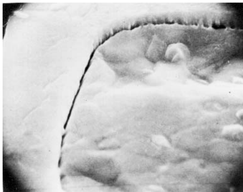
FIGURE 2077-11. Separation of metallization at contact step at 7,000X (reject)
