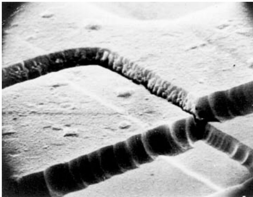
FIGURE 2077-13. Crack-like defect at oxide step at 7,000X (reject).
