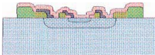
FIGURE 2072-9. Metallization misalignment, cross section view.
