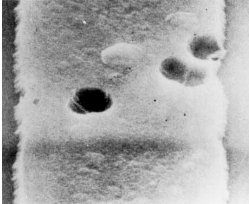
FIGURE 2077-20. General metallization voids at 5,000X (reject).
