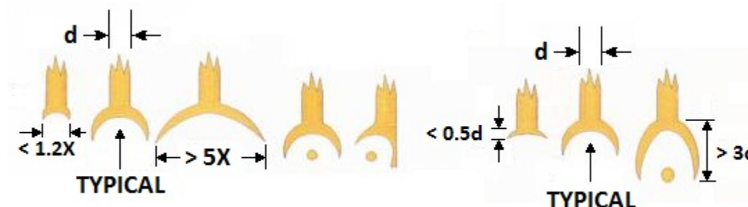
FIGURE 2072–23. Tailless bond dimensions.
