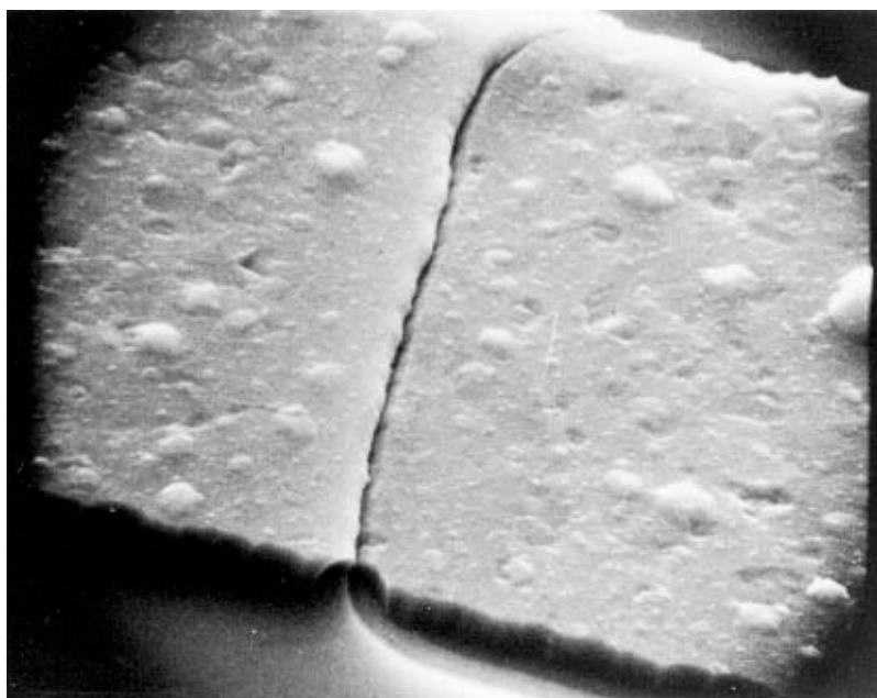
FIGURE 2077-9. Tunnel/cave at oxide step at 5,000X (reject).
