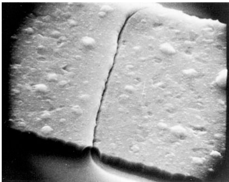
FIGURE 2077-9. Tunnel/cave at oxide step at 5,000X (reject).
