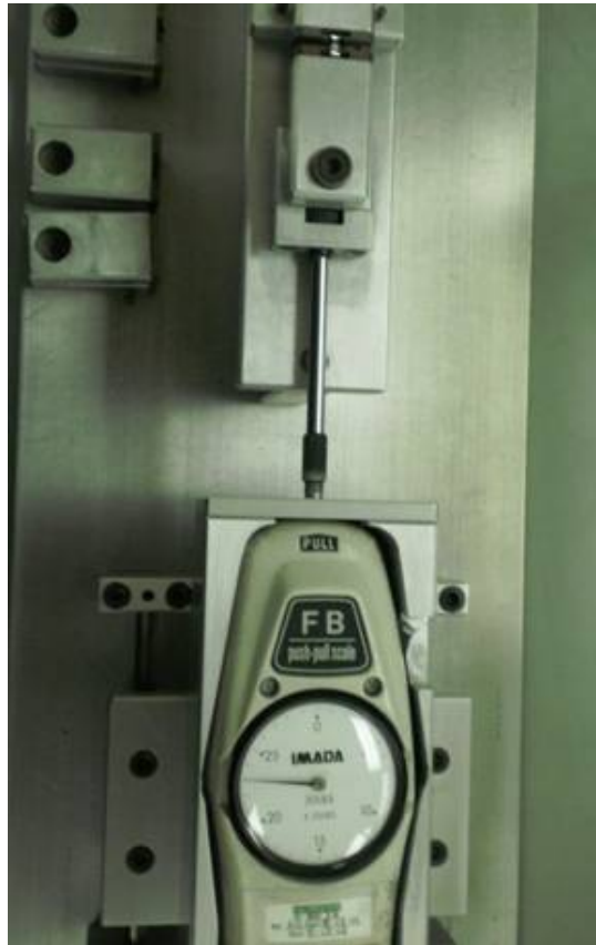
FIGURE 2038-1. Sample apparatus fixture with force measuring gauge.
