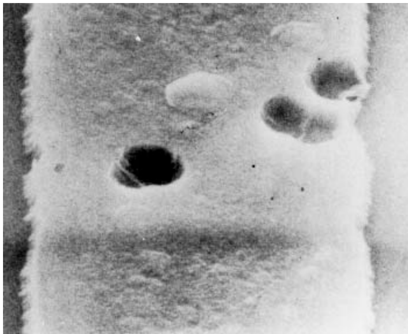
FIGURE 2077-20. General metallization voids at 5,000X (reject).
