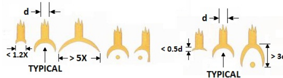
FIGURE 2072-23. Tailless bond dimensions.
