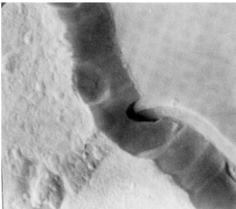
FIGURE 2077-8. Tunnel/cave at oxide step at 10,000X (accept).
