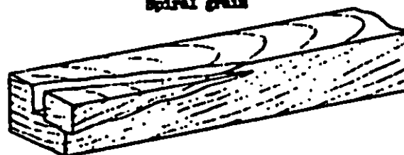
Spiral and diagonal grain in combination
