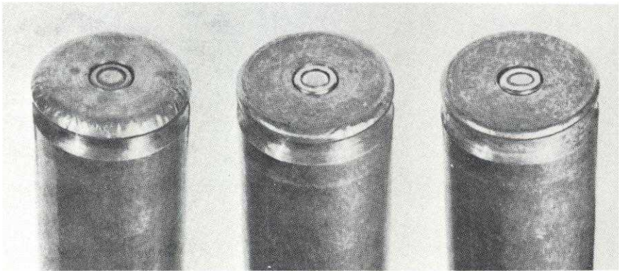
[.....Nonacceptable.....] [.....Acceptable.....] (round head)
