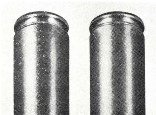
[ ..... Nonacceptable ..... ] [ ..... Acceptable ..... ] (Beveled underside of head)
