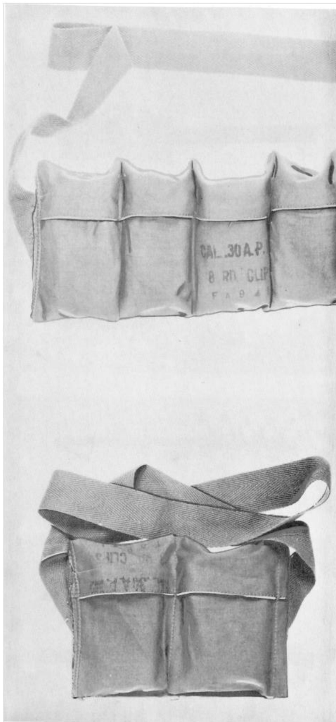
FIGURE A-58. Bandoleer package defect #1 – incorrect or illegible identification of bandoleer contents.
