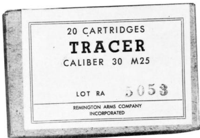
FIGURE A-3. Carton package defect #5 – misplaced or missing label, or improperly sealed carton.
