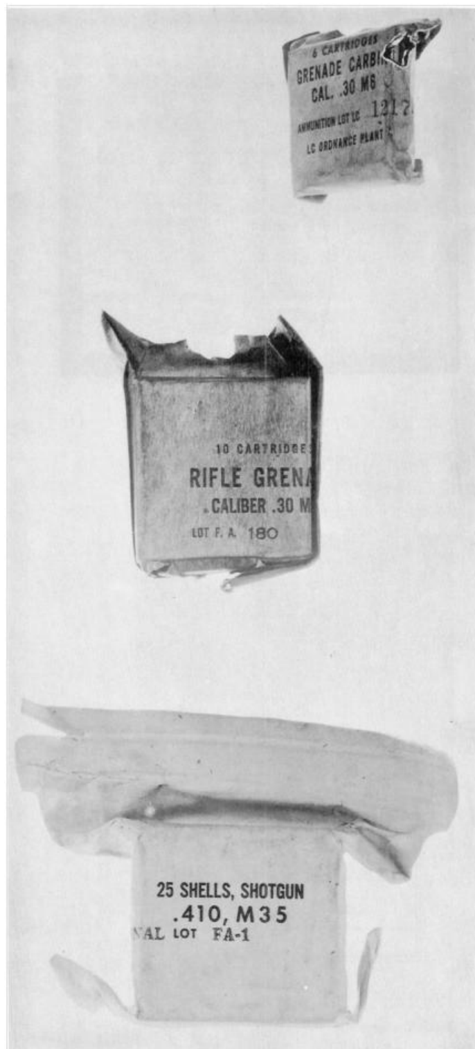
FIGURE A-15. Waterproof envelope package defect #1 – torn, ripped or improperly sealed envelope.
