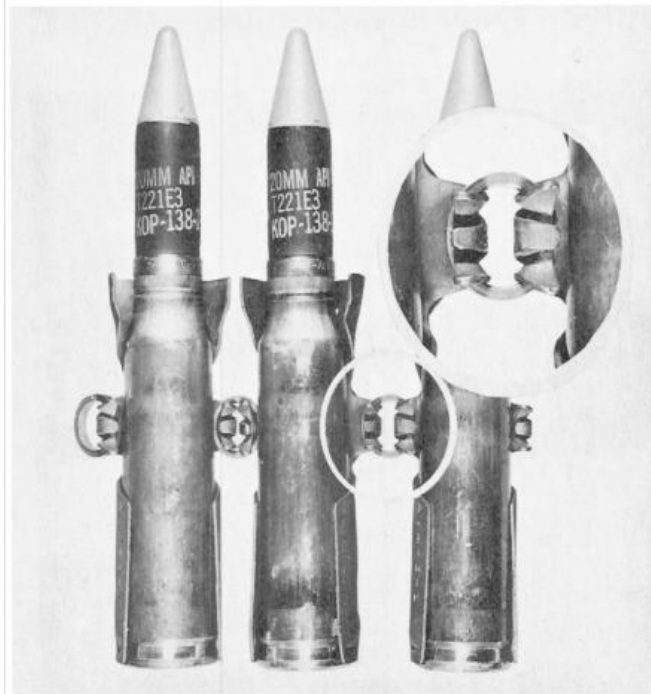
B – Unacceptable – Stretched link connecting ring.
