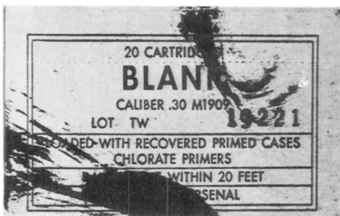
FIGURE A-13. Carton package defect #8 – incorrect or illegible identification of carton contents.
