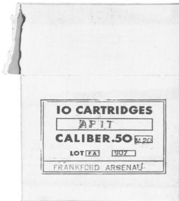
FIGURE A-9. Carton package defect #6 – torn or ripped carton or label.
