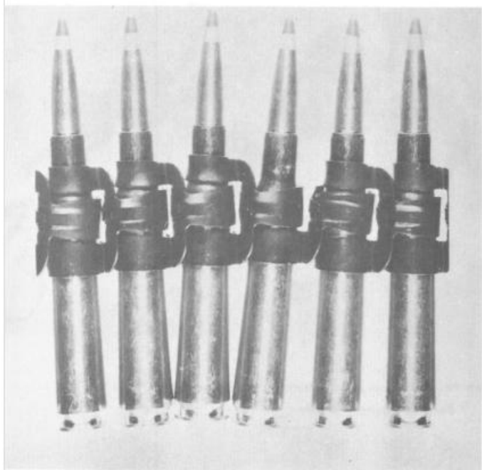
FIGURE A-34. Metallic linked belt package defect #5 – stretched, broken or “frozen” belt.
