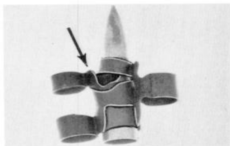
C – Unacceptable – Foreign matter Pronounced foreign material; some of cartridge body not shown.
