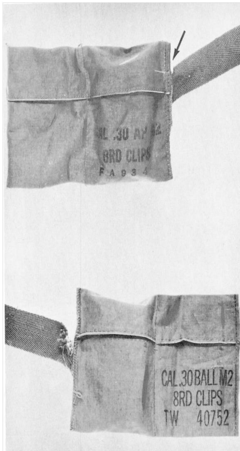
FIGURE A-63. Bandoleer package defect #3 – torn, ripped or otherwise defective bandoleer.
