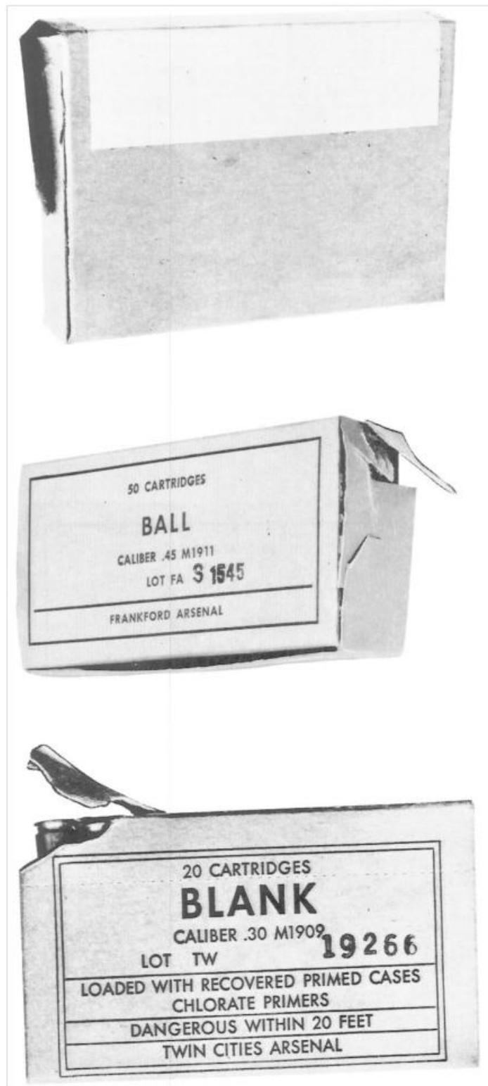
FIGURE A-10. Carton package defect #6 – torn or ripped carton or label.
