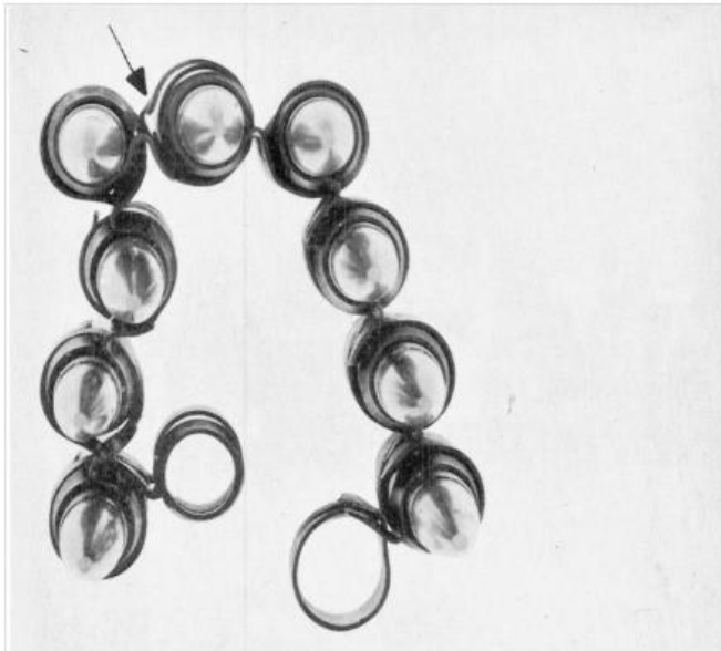
A – Acceptable – Stretched link connecting ring.
