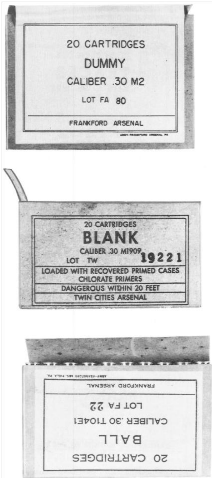
FIGURE A-6. Carton package defect #5 – misplaced or missing label, or improperly sealed carton.
