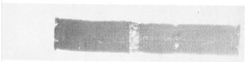
FIGURE A-67. Bandoleer package defect #3 – torn, ripped or otherwise defective bandoleer.
