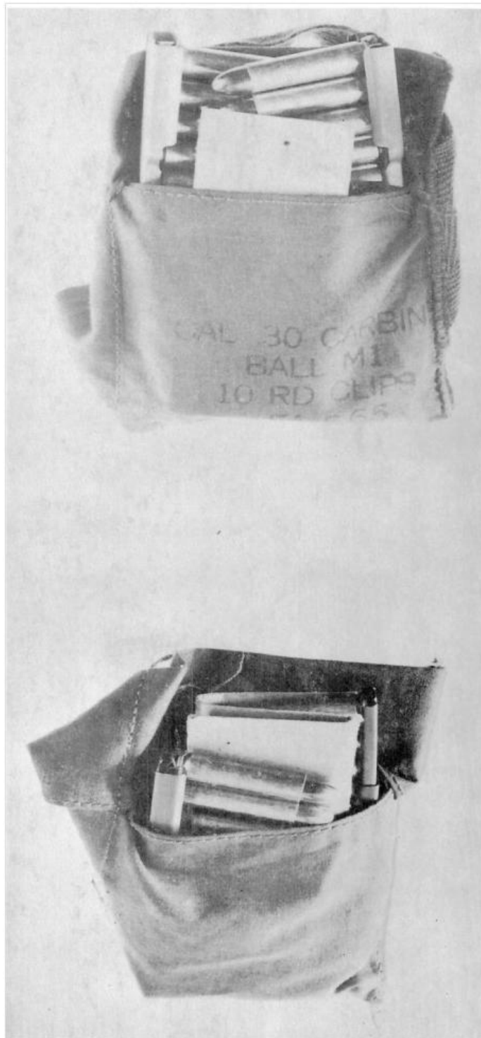
FIGURE 70. Bandoleer package defect #8 – improper packaging of clipped ammunition in bandoleers.
