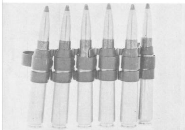
FIGURE A-48. Metallic linked belt package defect #8 – malformed link(s) – pronounced.
