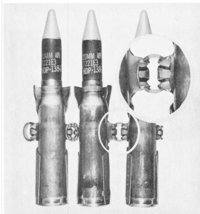
B – Unacceptable – Stretched link connecting ring.
