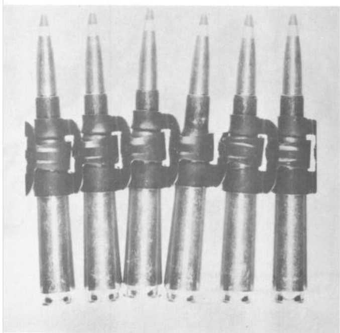
FIGURE A-34. Metallic linked belt package defect #5 – stretched, broken or “frozen” belt.
