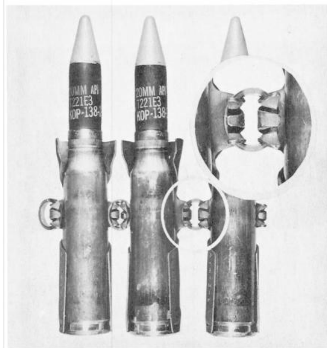
B – Unacceptable – Stretched link connecting ring.
