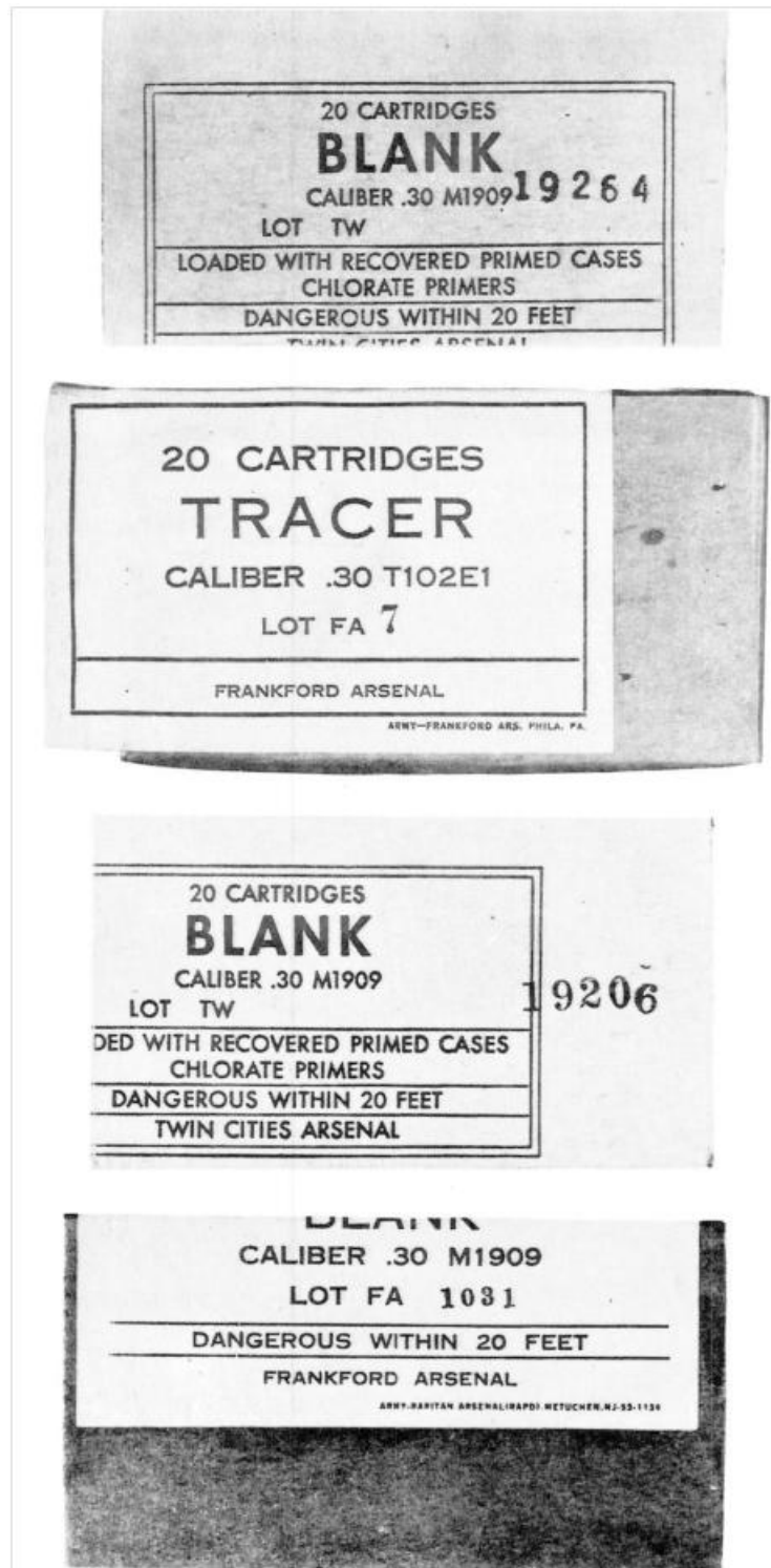
FIGURE A-4. Carton package defect #5 – misplaced or missing label, or improperly sealed carton.
